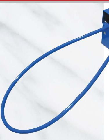
This unit can be easily mounted on the side of virtually any machining center coolant sump. By use of an existing opening or by making a small access cutout, the collector tube runs through the surface of the coolant and collects the unwanted oils. The oil then flows out the discharge tube into any waste oil container for easy disposal.
