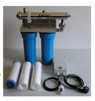
Save disinfection by UV light requires that the treated water has a good UV transparency and is free of particles and turbidity. This is achieved by prefiltration. The compact type unit ABOX®WAS combines the prefiltration and the UV disinfection in a common device. The compact and space saving design is making it ideal for using on boats, in holiday houses or shelters or for mobile applications.
